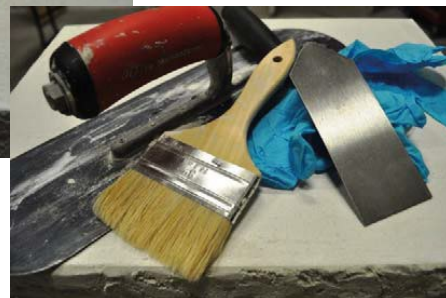
Tools Needed for Trowel Coats: Gloves, Chip Brush, Margin & Pool Trowel
