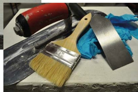
Tools Needed for Trowel Coats: Gloves, Chip Brush, Margin & Pool
